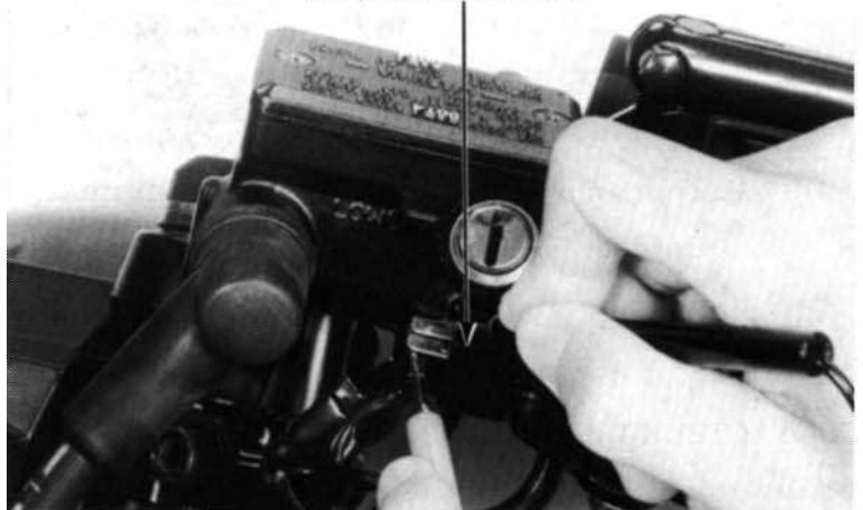
(2) CLUTCH APPLIED: CONTINUITY CLUTCH RELEASED: NO CONTINUITY
